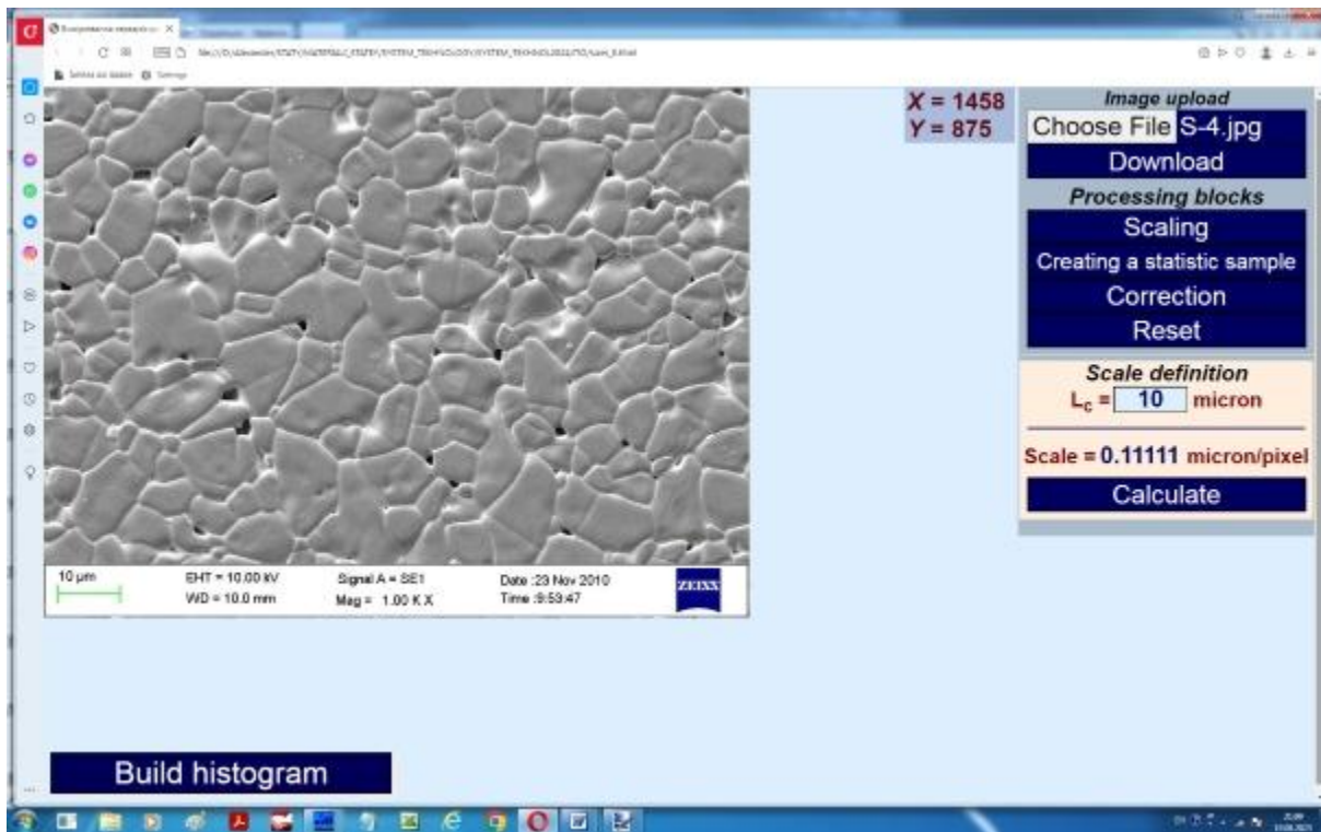
Figure 2 - Web page of program at the final stage of bitmap scaling
