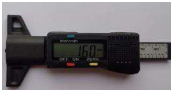
Figure 2 - Digital tread depth sensor
