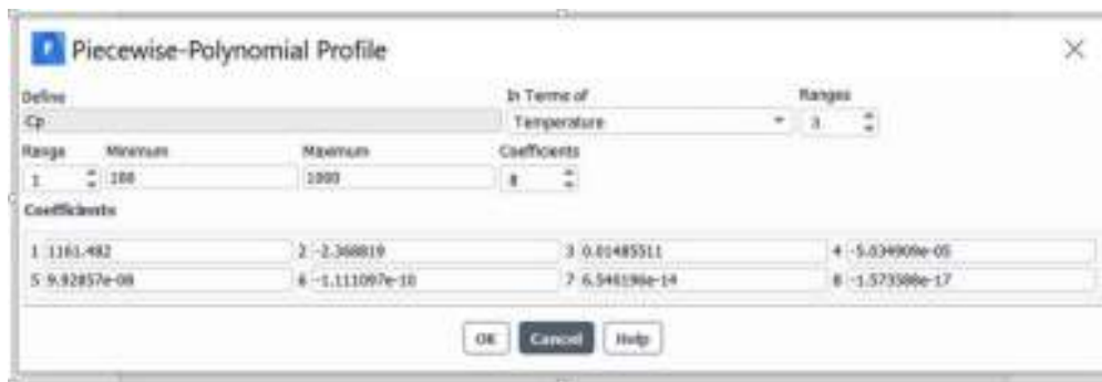
Figure 2 - Setting the approximating formula for thermal conductivity in the ANSYS software package
