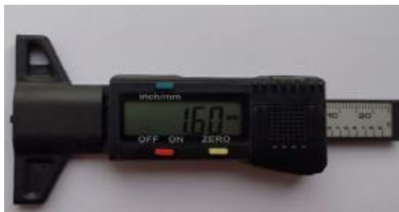
Figure 2 - Digital tread depth sensor
