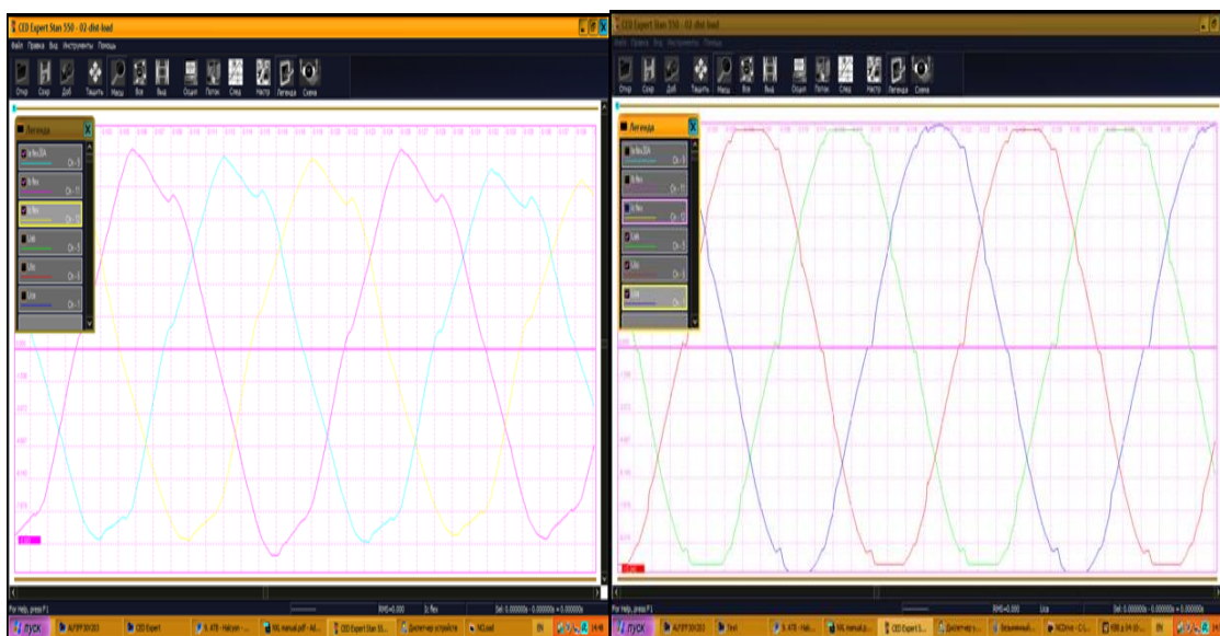
Figure 4 - Oscillograms of currents (from above) and voltages (from below) within the considered electric motor while operating under loading
