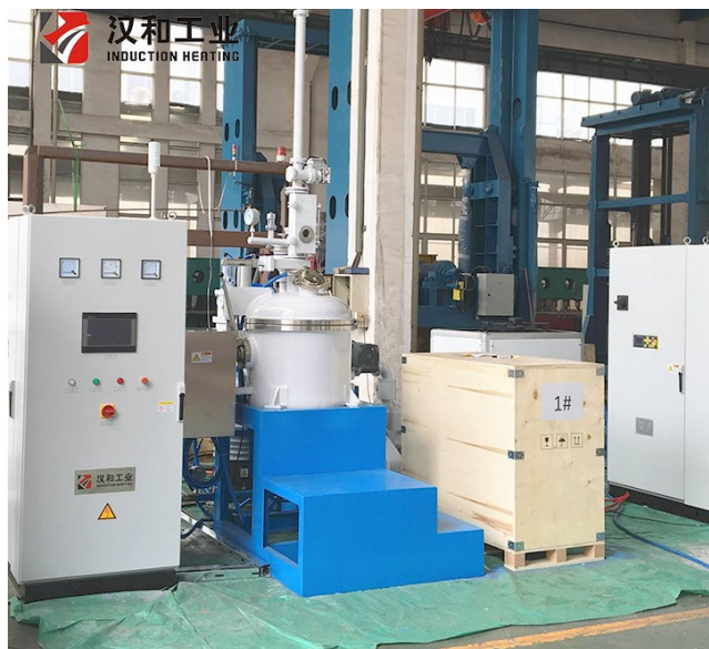
Figure 2 – Vacuum induction furnace of the company Zhuzhou Hanhe Industrial Equipment Co., Ltd. [26]
