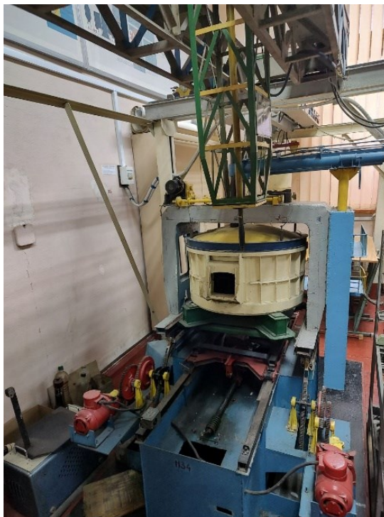
Figure 1 – Model of an electric arc furnace with a rolling hearth in the laboratory of the Department of Metallurgical Equipment of Zaporizhzhia National University
